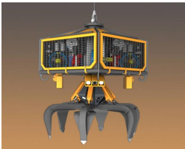
Fig 3 UTROV Grabber system for boulder removal
