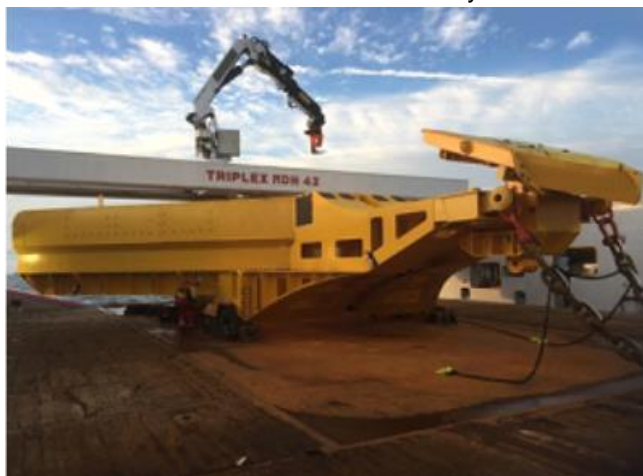
Fig 2 Ecosse Subsea Systems 15m SCAR Plough
