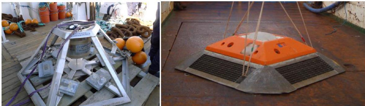
Fig. 6 Acoustic doppler current profilers
